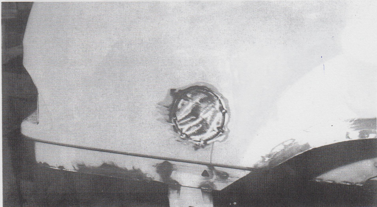
If a Ford-supplied safety bag fuel tank is to be fitted, the existing SIERRA fuel filler access becomes redundant. A closing panel should be welded into place.
